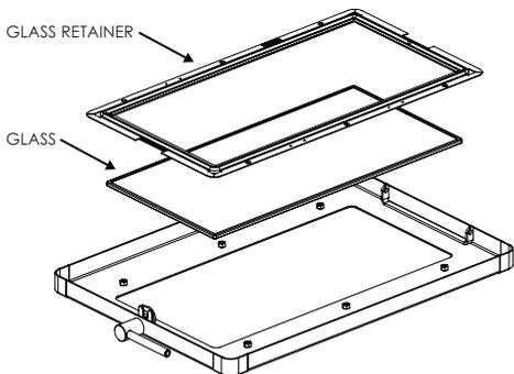
3. Flip the retainer over, remove the old glass.
