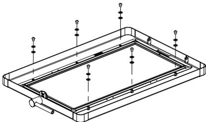
2. Gently lift the glass retainer up and out, taking careful note that the glass may still be held in the retainer and could fall out.
